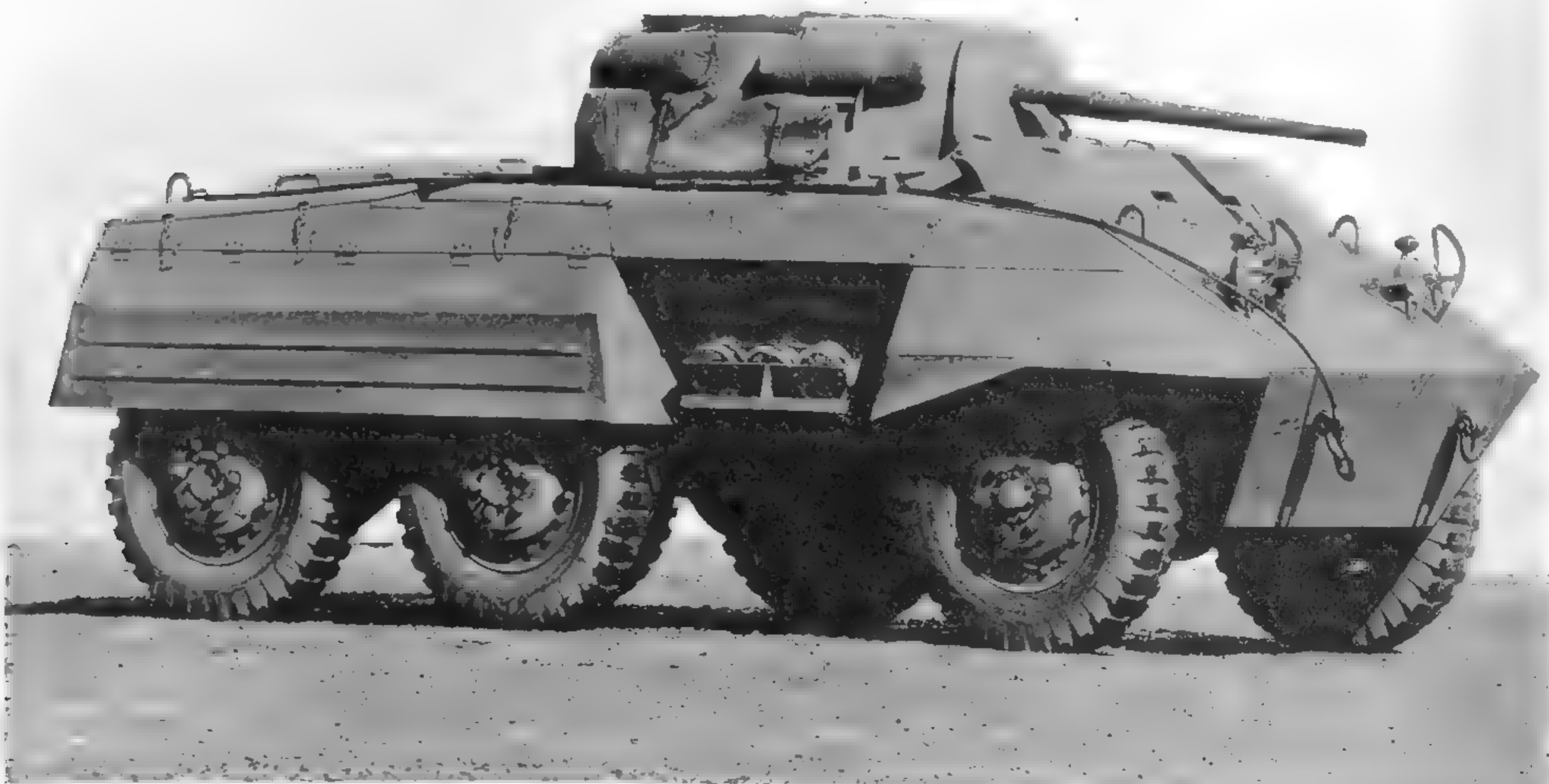
The M8 was armed with a 37mm gun in its turret from the outset, and later models added a .50-caliber machine gun on the turret as well. This is an early vehicle, as evidenced by the mine rack on it side. (U.S. Army photo)
